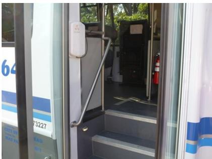
Front RFID antenna in paratransit bus
